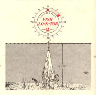
Weeds don't grow in water more than 12 to 15 feet deep in most lakes because of the lack of sunlight. They make a great many thin, pale signals on the FISH LO-K-TOR dial. As the boat approaches underwater weeds the faint signals climb up toward the zero signal; as the boat leaves, they go back down the dial toward the bottom signal. You will also observe these same climbing and descending signals as your boat approaches and leaves trees or brush. Their signals are brighter.
