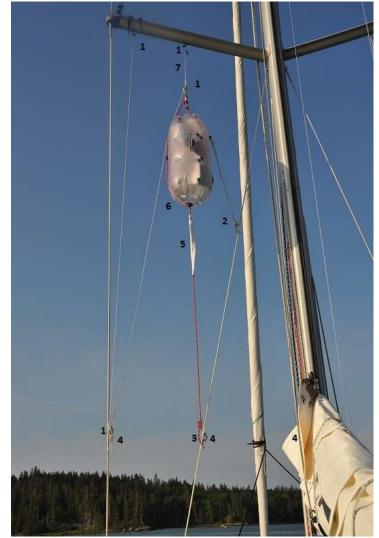
the shroud above each cleat I have wrapped rigging tape, to prevent the snap hook (3) from rubbing the shroud (noise reduction). Each of these points are equal distance from above, so that I can unclip and move it to another attachment point without adjusting the flag halyard.
