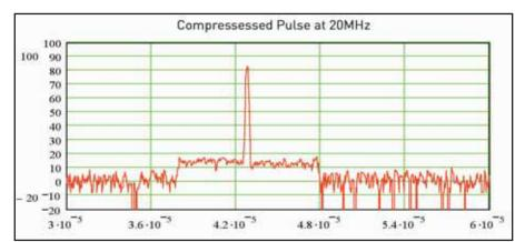
0.05%. To ensure detection performance is unimpaired, the system transmits longduration pulses, equalling or surpassing the pulse energy obtained from a magnetron. Fine-range resolution is maintained by encoding the long-duration pulses so that they can be compressed into narrow pulses by digital signal processing techniques employed in the radar receiver.
